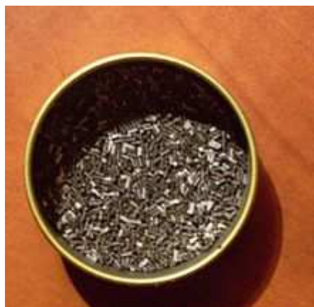
Poudre B single-base smokeless powder flakes
