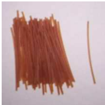
Sticks of cordite from a .303 British rifle cartridge.
