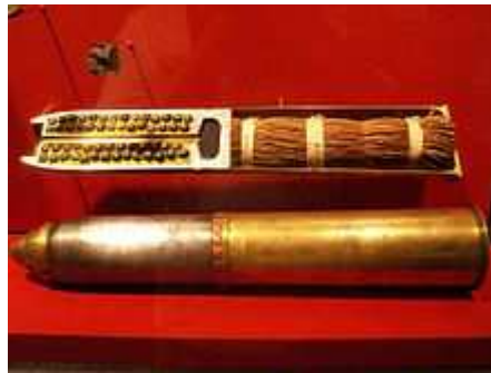
A sectioned British 18 pounder field gun shrapnel round, World War I, showing string bound to roughly simulate the appearance of the cordite propellant
